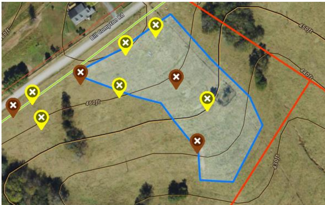
Figure 4. Usable area for a conventional septic system.
