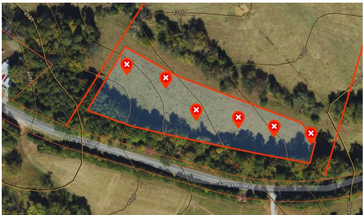
Figure 4. Usable area for a conventional septic system.
