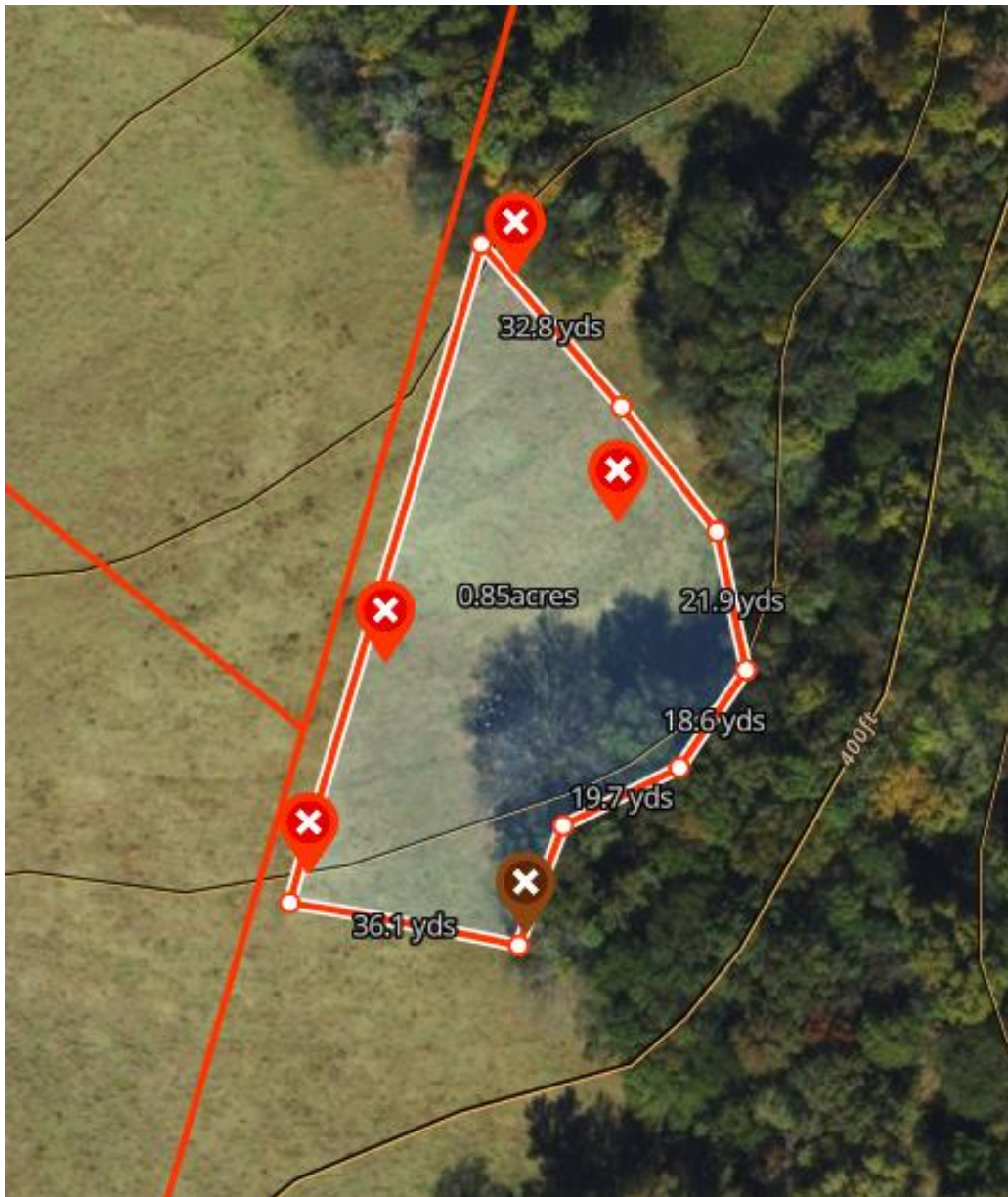
Figure 4. Usable area for a conventional septic system.
