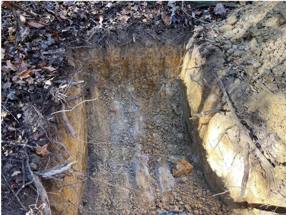
Figure 7. Cid soil with hard slate present at the bottom of the pit.
