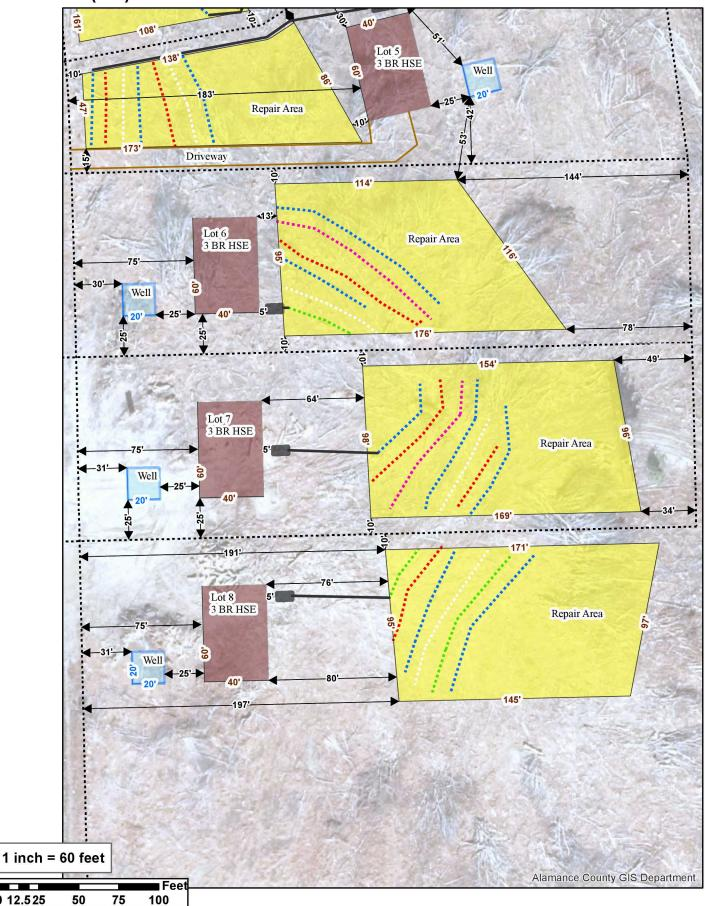
Scale is approximate and may not be accurate on emailed, scanned, and faxed copies of this drawing.
